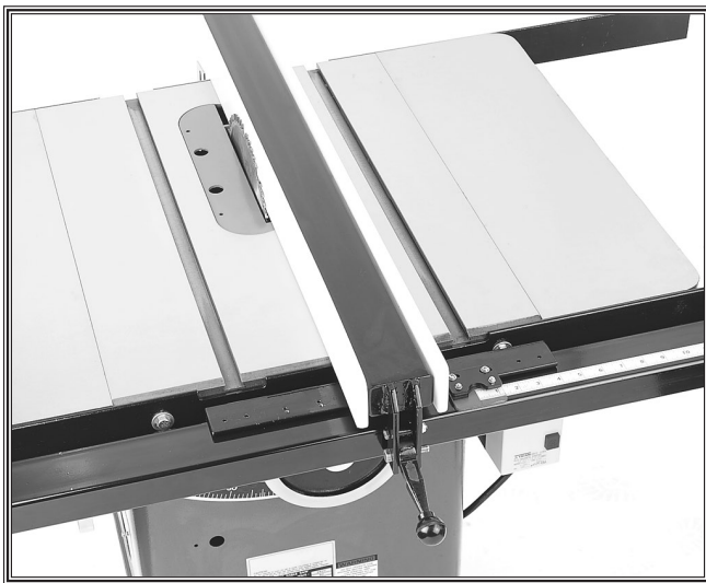
Figure 12. Fence contacting the blade.
